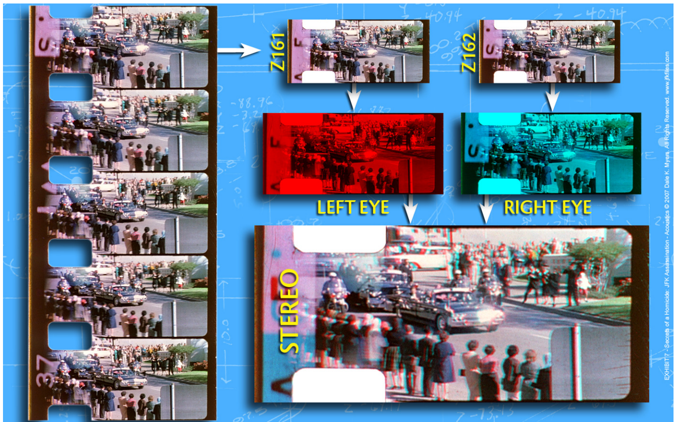
Exhibit 7. Process of creating stereoscopic images from adjacent film frames.
