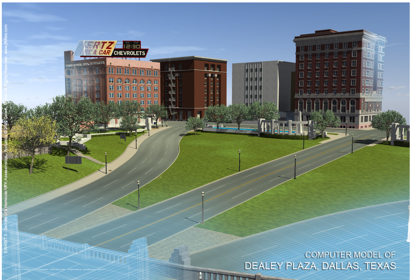
Exhibit 3. Computer model of Dealey Plaza based on survey maps, blueprints, photographs, and measurements.
